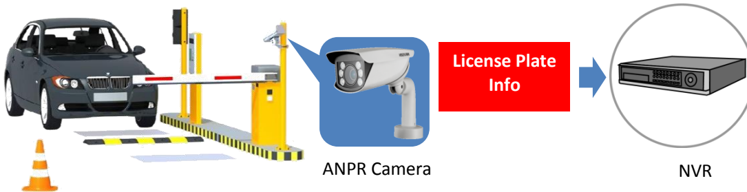
Figure 3-10 NVR+IPC Solution Mode
